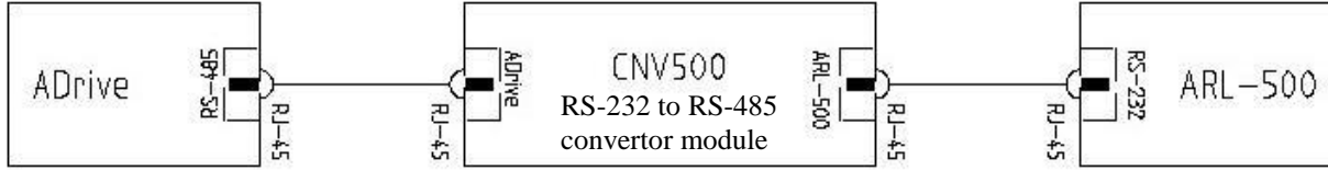
Serial communication with ARL-500
