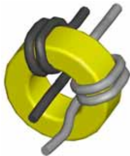
Toroidal core in BR09-1 and BR11-A
